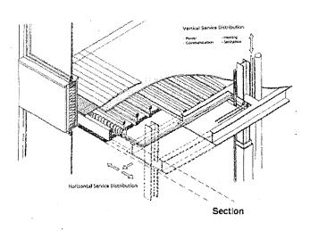
Fig. 2. Competition Proposal for the Modular Service Core. Note the service trench formed by the two beams and the construction of the floor cassette.
