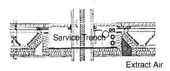
Fig. 4. Section through the service trench/floor cassette. The small area used for the ventilation ducting can be seen adjacent the steel W sections.
