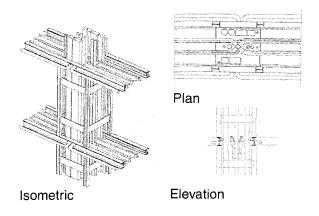
Fig. 3. Isometric, Plan and Elevation of the Scheme Design Core. With all services preinstalled. Prefabricated Cores.
